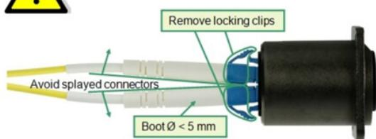
Avoid splayed connectors by using LCs without anti-snag collars and a boot diameter < 5 mm (available from suppliers as e.g. Corning).
