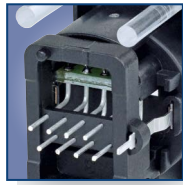
Vertical PCB with lightpipes
